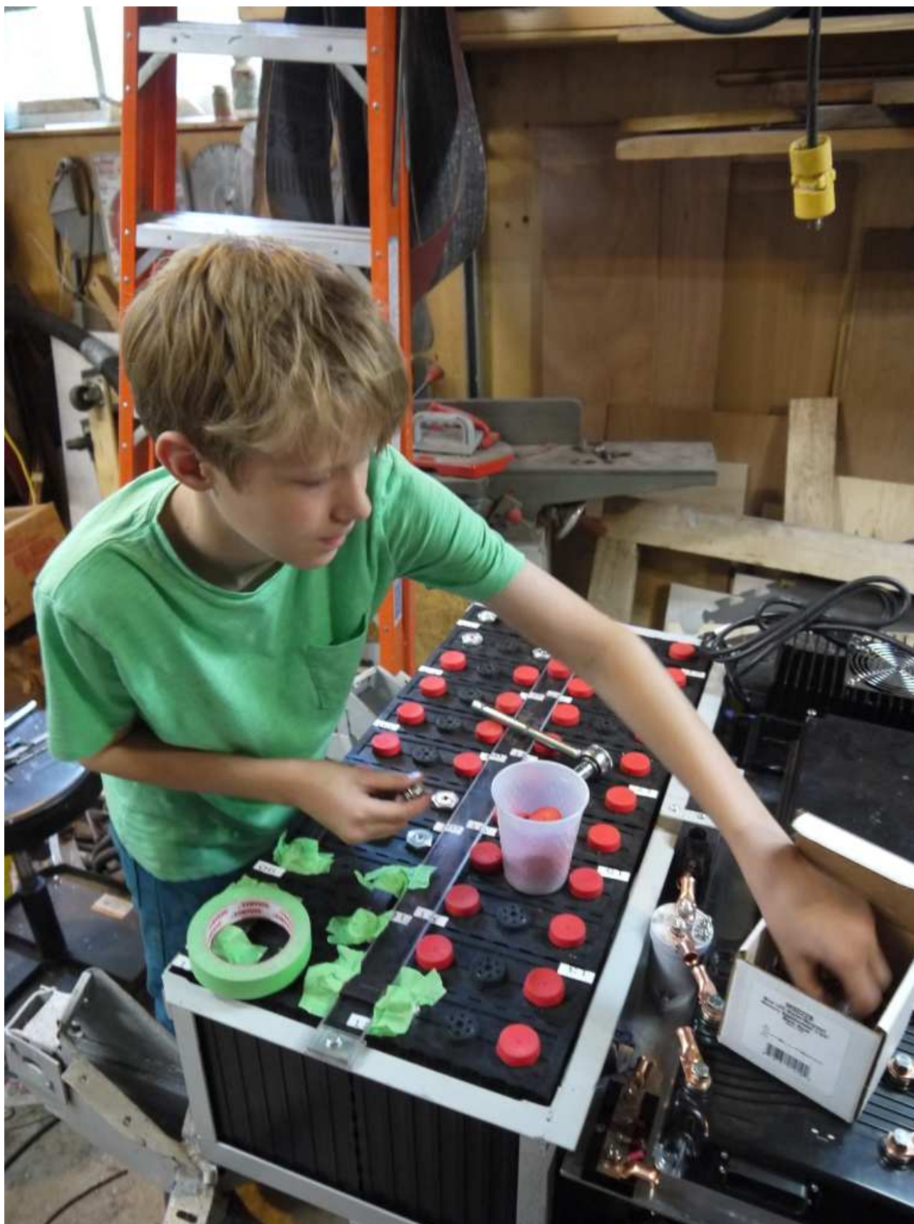
Jacob wiring the front battery pack– 22 LiFePO4 180Ah batteries.
