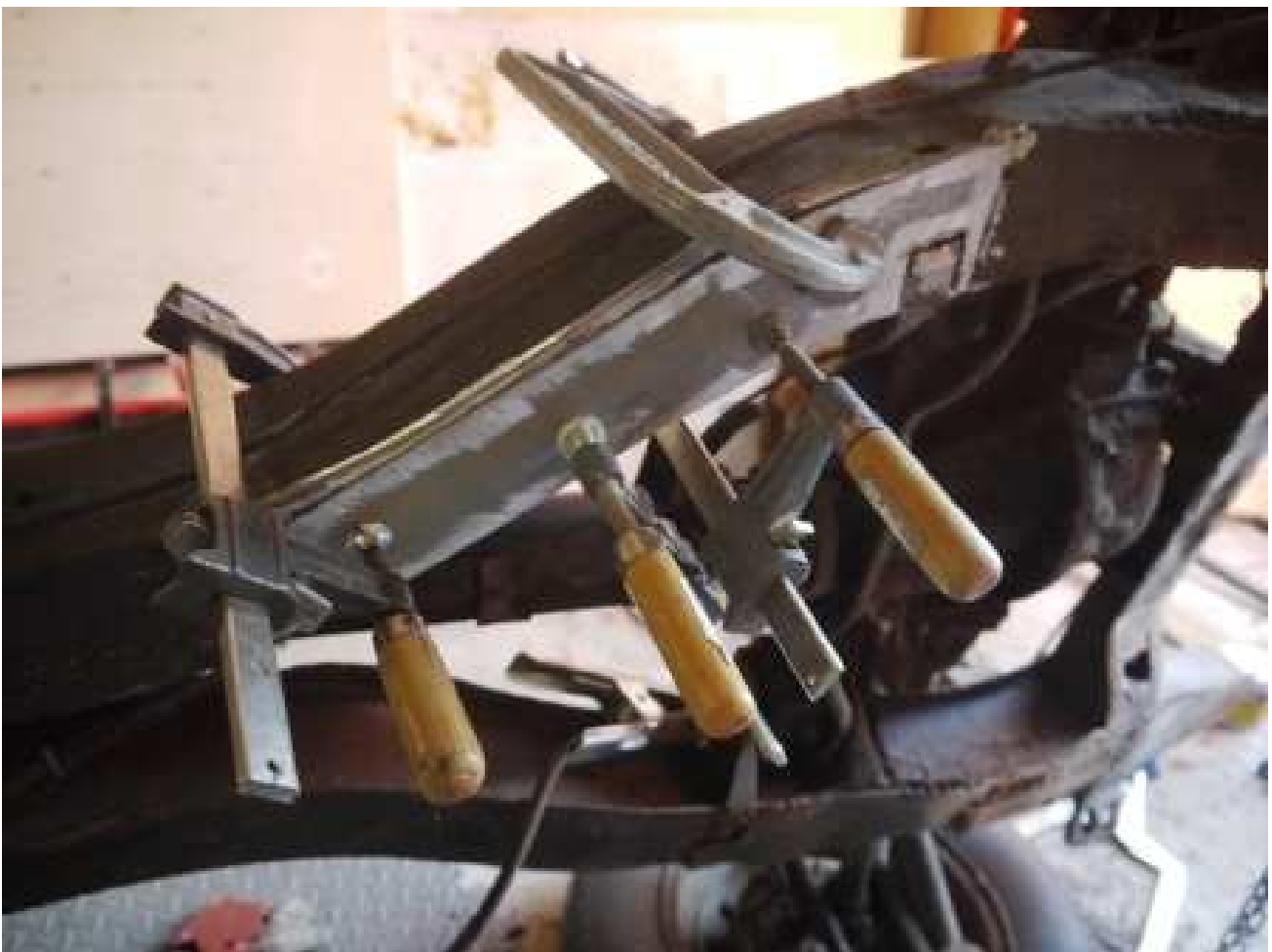
Parts of the frame/chassis were rusty enough to need reinforcement.
