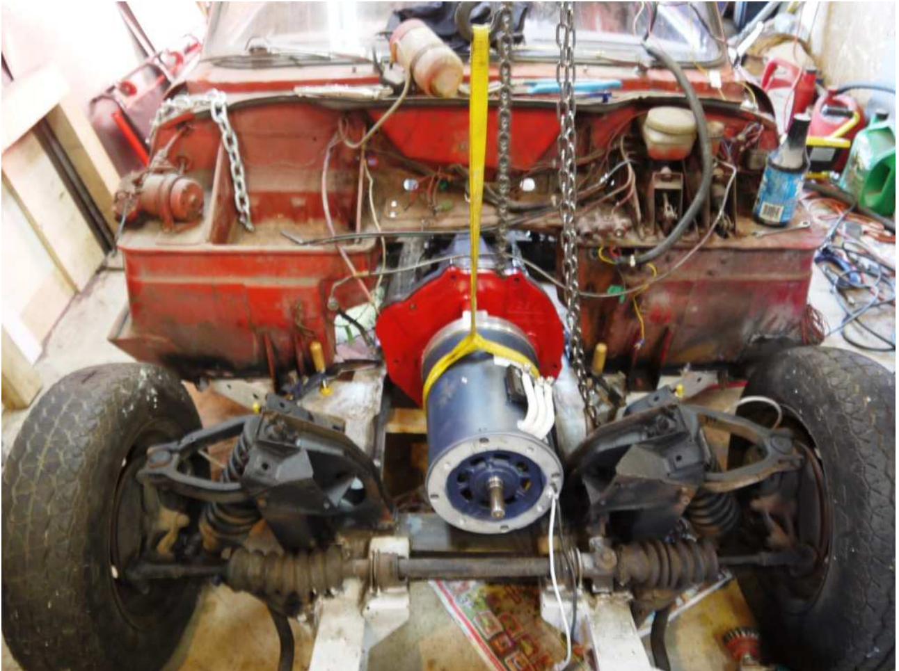
The AC-50 motor (blue/silver) bolted to the CanEV transmission mounting plate (red).
