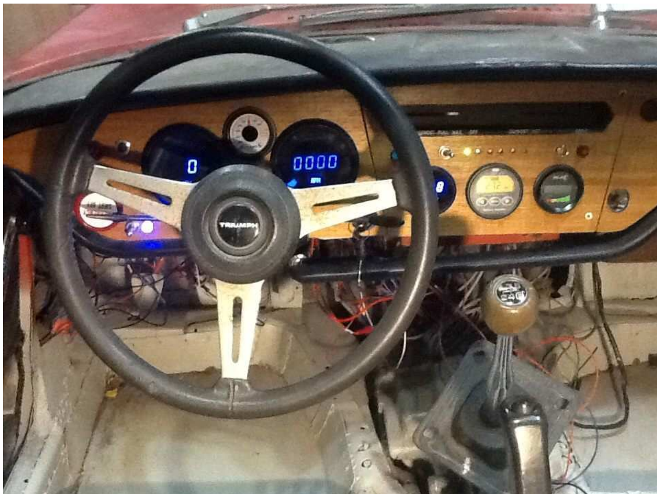
The dash and re-wiring in progress— a wooden dash not only gives a lovely look, it makes re-building a lot easier. The white gauge nestled between the speedo and tach is the ammeter, which measures battery current both forward (during driving) and reverse.
