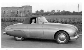
The front track width was too narrow and this was creating problems in the tapering of the body in the rear section, with the risk to have the front wheels "disappear" below the fenders. But this
