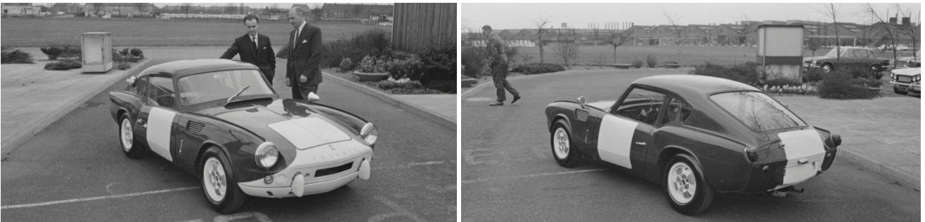
The first prototype of the Works Spitfire used for the tests before the participation to the 24 Hours Le Mans in 1964: the hardtop is the copy in fiberglass of the one designed and built in Turin by Michelotti for the Spitfire Gt and proved to have a significant aerodynamic efficiency, while the bonnet is still without the headlamp fairing.
