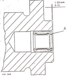
The procedure for fitting the needle roller bearing is as follows:
