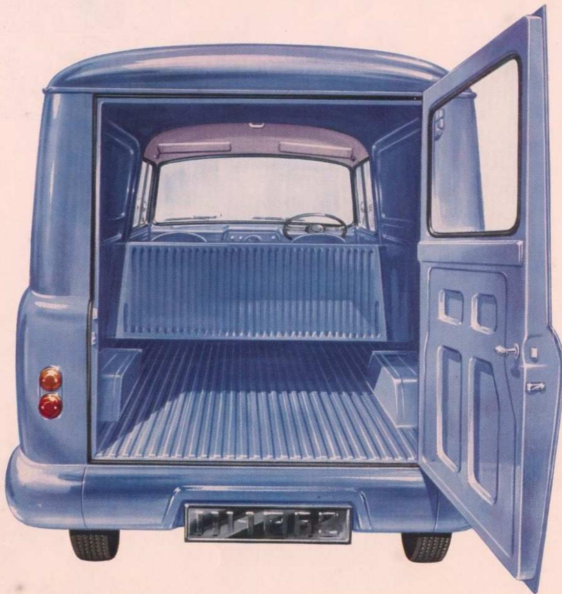
The ATLAS MAJOR packs a load of 180 cu. ft.—all on a 7 ft. wheelbase. This is a greater capacity than any other vehicle with a similar payload. The main goods compartment is 92" long, 63" wide, 55" high. There's additional space beside the driver when no passenger is carried.
